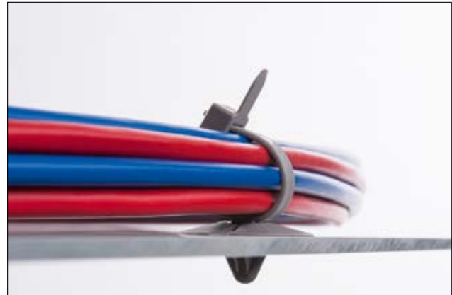
T80RSFT - The 'tab' on the head of the tie makes it easy to locate and lift the head for assembly.
