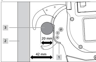
The distance from front cap 1 to flat 2 must be at least 42 mm. Bundle 3 can be no more than 20 mm in diameter.
