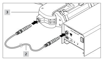
Use connecting cord 2 to connect the power pack to tool AT2000 CPK 3.
