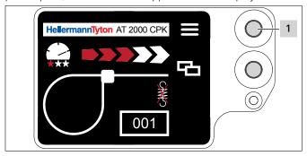
Enter button to confirm a selection in the navigation menu and increment switch for display menu settings
