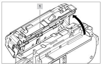
Serial number 1 is inside the AT2000 CPK. It is visible when the gate is open.
